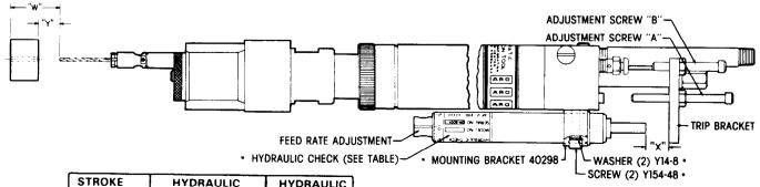
**HYDRAULIC** CHECK ASS'Y **LENGTH** CHECK NO. 1 INCH 40301-2 38922 INCH 40301-3 38922-1 3 INCH 40301-4 38922-2
